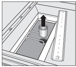
■ Remove the fine filter and clean if necessary.
